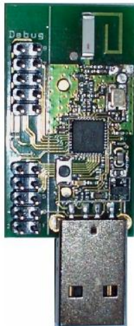
Figure 34. Chip Antenna from Johanson Technology for 868/915/955 MHz
